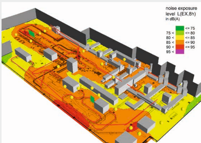
Noise exposure level in a factory hall
