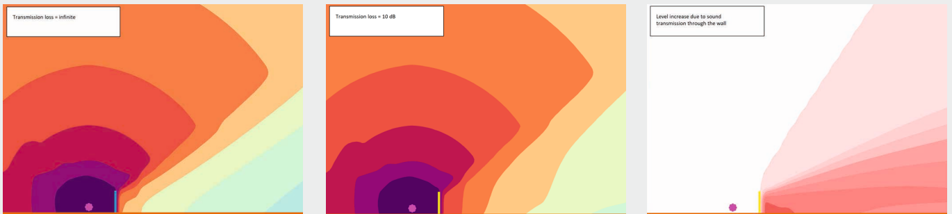
The figure on the left shows the shielding due to a wall calculated according to ISO 9613-2:2024 with an infinite transmission loss. The middle image shows the results with an assumed transmission loss of 10 dB, and the right image shows the difference between the two calculations (scaled in 1 dB steps).
